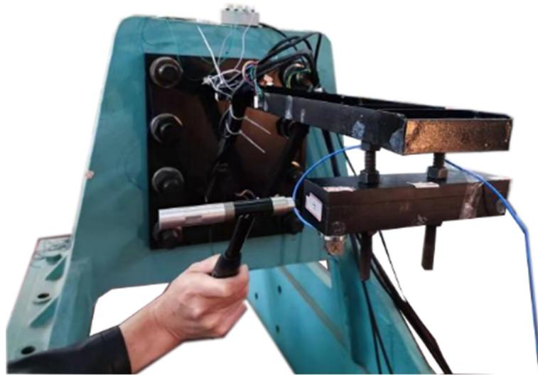
Figure 4. Test of single pylon.
