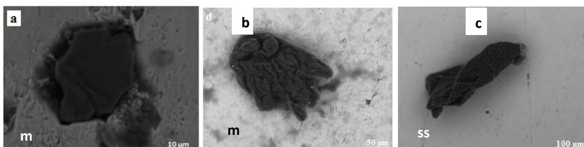
**Figure 4.** Smooth and wrinkled matrix surface topographies of 7 days old biofilms formed in non-diluted milk (a and b) and nutrient broth (c) by *B. cereus* strains S78 (a), A7 (b) and P56 (c). (m) Indicates milk fouling coating stainless steel surface topography and (ss) stainless steel.
