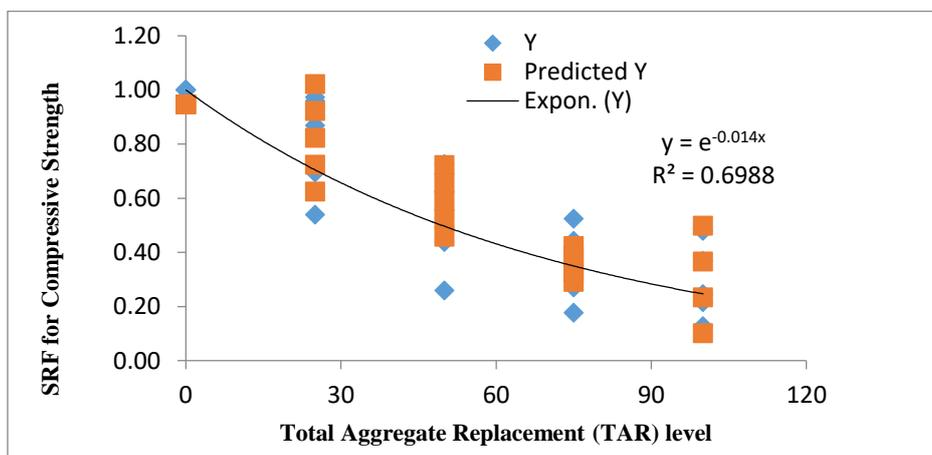
Fig. 1. Relationship between SRF for compressive strength and TAR
