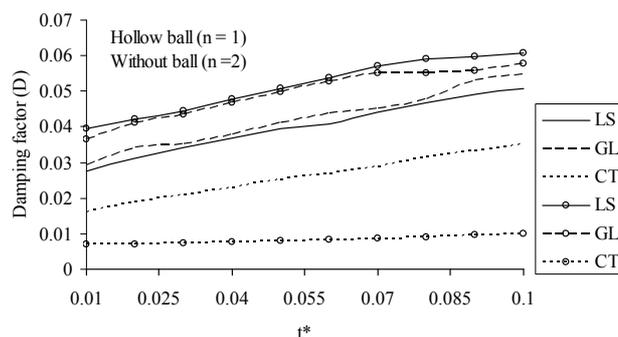
**Figure 6.** Variation of damping factor with thickness to mean radius ratio for different values of degree of spherical harmonics ( $n$ ) for helium material in case of rigidly fixed boundary condition.
