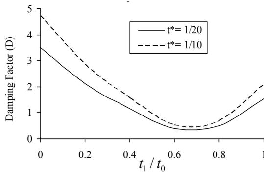
**Figure 12.** Variation of damping factor with time ratio for various value of  $t^*$  for magnesium material.
