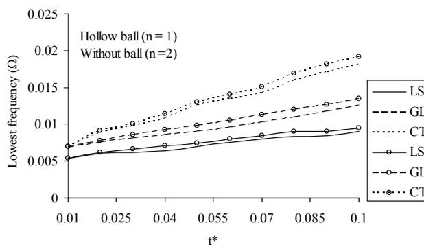
**Figure 5.** Variation of lowest frequency with thickness to mean radius ratio for different values of degree of spherical harmonics ( $n$ ) for helium material in case of rigidly fixed boundary condition.
