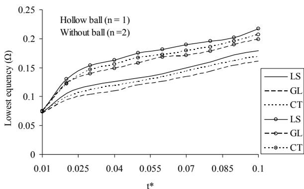
**Figure 3.** Variation of lowest frequency with thickness to mean radius ratio for different values of degree of spherical harmonics ( $n$ ) for magnesium material in case of stress free boundary condition.
