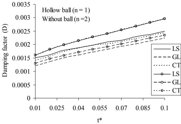
**Figure 8.** Variation of damping factor with thickness to mean radius ratio for different values of degree of spherical harmonics ( $n$ ) for magnesium material in case of rigidly fixed boundary condition.
