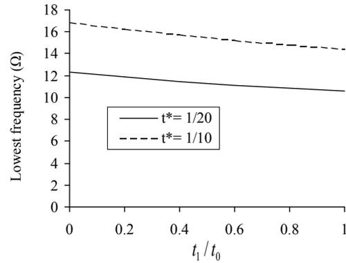
**Figure 9.** Variation of lowest frequency with time ratio for various value of thickness to mean radius ratio ( $t^*$ ) for helium material.
