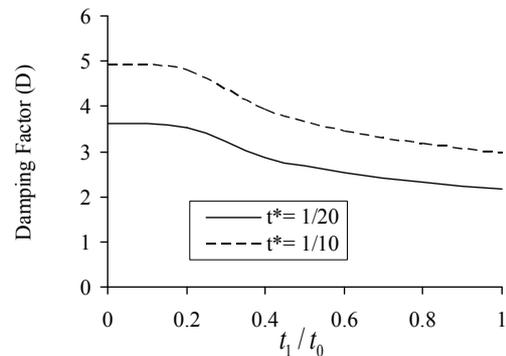
**Figure 10.** Variation of damping factor with time ratio for various value of  $t^*$  for helium material.
