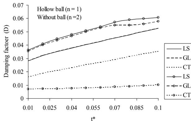
**Figure 2. Variation of damping factor with thickness to mean radius ratio for different values of degree of spherical harmonics ( $n$ ) for helium material in case of stress free boundary condition.**
