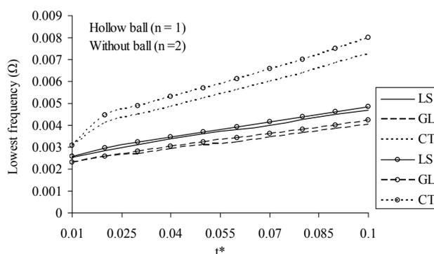
**Figure 7.** Variation of lowest frequency with thickness to mean radius ratio for different values of degree of spherical harmonics ( $n$ ) for magnesium material in case of rigidly fixed boundary condition.
