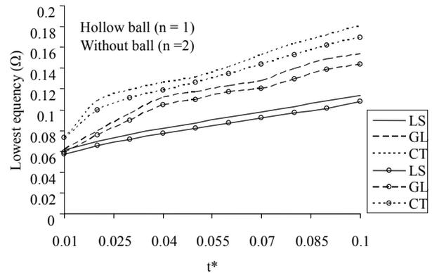
**Figure 1. Variation of lowest frequency with thickness to mean radius ratio for different values of degree of spherical harmonics ( $n$ ) for helium material in case of stress free boundary condition.**
