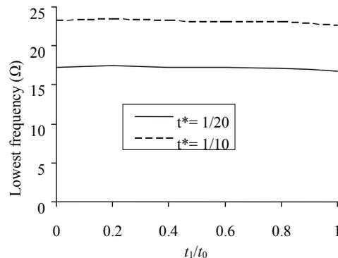
**Figure 11.** Variation of lowest frequency with time ratio for various value of  $t^*$  for magnesium material.
