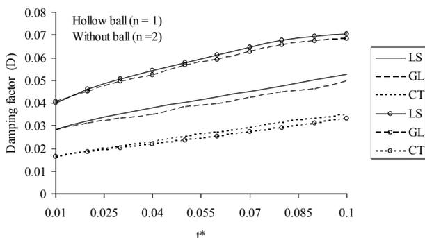
**Figure 4.** Variation of damping factor with thickness to mean radius ratio for different values of degree of spherical harmonics ( $n$ ) for magnesium material in case of stress free boundary condition.
